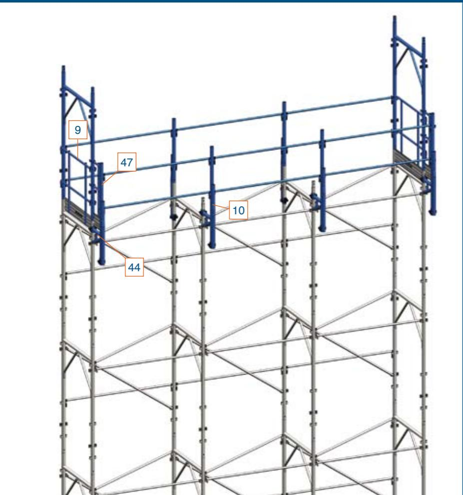
SCHEMA CON MENSOLA DA 0,600 m / STRUCTURE WITH BRACKET OF 0,600 m
